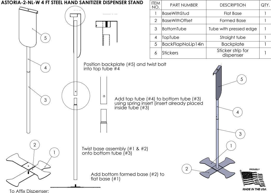
To affix dispenser to the Astoria Stand, please use the dual stick square stickers enclosed with this stand. Place stickers on each corner of the dispenser and across the top. Carefully position the dispenser flush to the top of the backplate and press firmly to secure.
