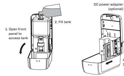
Ensure switch is in OFF position. Fill tank with liquid sanitizer. Turn switch to ON position to power on.
