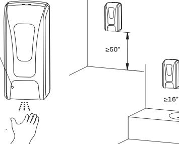
Position dispenser 8" minimum from surfaces to prevent false readings. Install out of direct sunlight and humidity.
