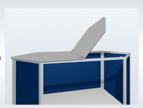
Unfold the top shelf and fix its position.
